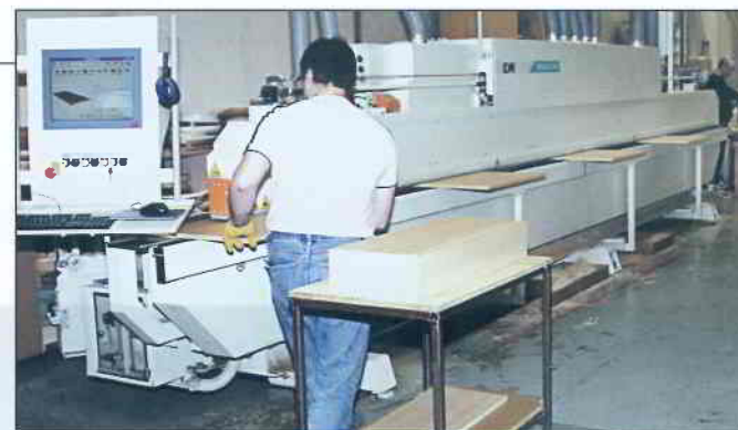
Dave runs the edge finishing show on his own at Holz Mobil and has his work cut out manning both ends of the new IDM Genesis from MSL at the same time.
