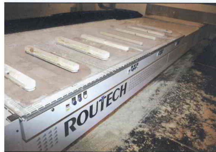
Four head Routech is turning out 2,000 seat back components in a two-session compared with 200/wk by previous methods.
