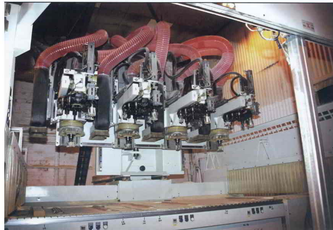
Four heads working pendulum style, the Bradford factory has instantly doubled output of the best-selling products.
