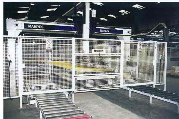
Since supplying the Morbidelli Author 660, Machine Sales has also supplied the Mahros Runner panel stacker on the end of the line at the Ashcraft Furniture factory.
