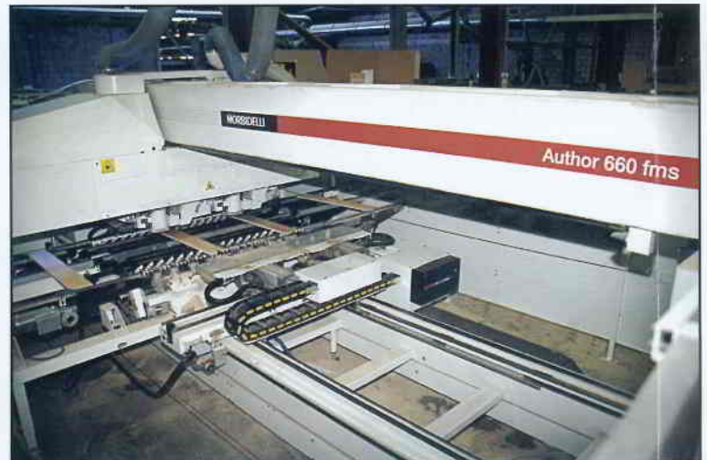
Shown point-to-point drilling, routing and grooving narrow rails in a single pass is the Morbidelli Author 660 from Machine Sales at Ashcraft Furniture.
