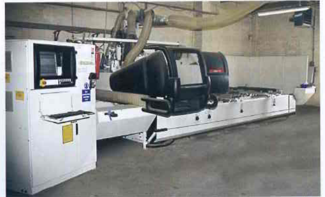
Both the Author 744S and the new Planet Super share Morbidelli's Rapid auto tool changer technology
