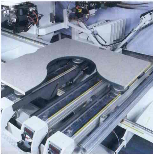
Planet Super carries new photo-electric cell technology for edge finishing shaped workpieces to very high standards of precision
