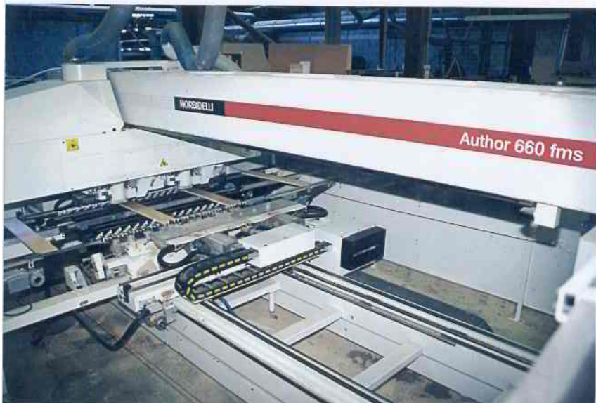
Shown point-to-point drilling, routing and grooving narrow rails in a single pass is the Morbidelli Author 660 from Machine Sales at Ashcraft Furniture
