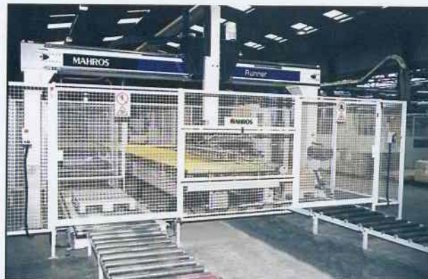
Since supplying the Morbidelli Author 660, Machine Sales have also supplied a Mahros Runner panel stacker on the end of the line at the Ashcraft Furniture factory.
